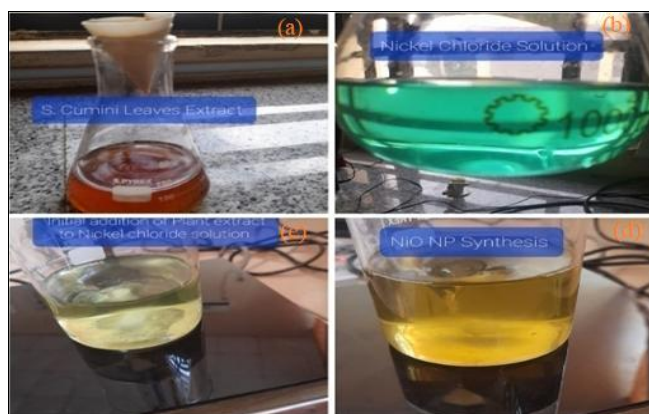
Plate 3: Colour changes for the synthesis of nickel oxide nanoparticles.
