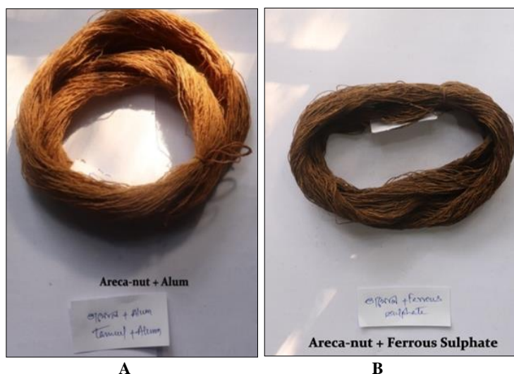
Fig 1: Eri silk-yarn died with extraction of Areca nut and Alum mordant (A), Areca nut and Ferrous sulphate mordant (B)
