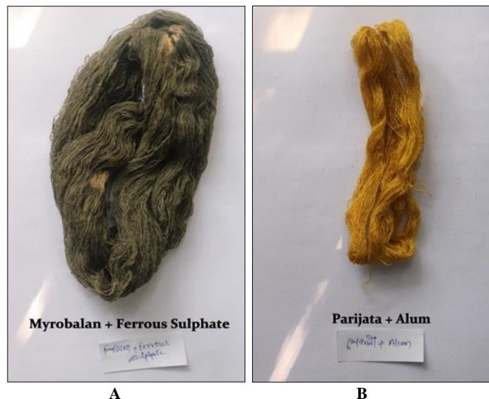
Fig 3: Eri silk-yarn died with extraction of Myrobalan and Ferrous sulphate mordant (A), Parijata and Alum mordant (B)
