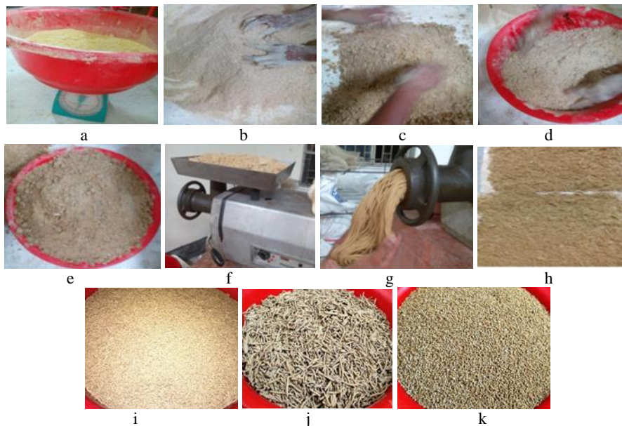
Fig 1: Flow diagram for preparation of Diet-2 (Formulated feed with pangas waste) and other two Diets (where, a-rice bran; b-dried powder of pangas processing waste; c-mixing of ingredients; d- addition of water to the ingredients; e-paste of ingredients; f-ingredients in mincer; g-fed pellet preparation; h-drying of feed pellets; i-Diet-2 (diet with pangas waste); j-Diet-3 (diet without pangas waste); k-Diet-1 (commercial diet)
