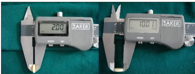
Fig 2: Dimensions measured of prepared porcelain specimen.
